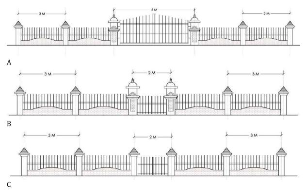
Figure 31: Details of Proposed Boundary Walls (A - with Vehicular Entry; B - Primary Pedestrian Entry; C - Secondary Pedestrian Entry)
